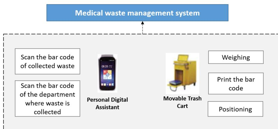
**Figure 4.** Illustration of medical waste management system by Ewell.
