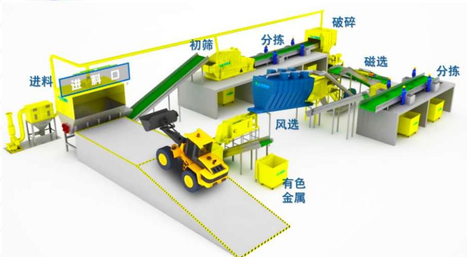
Picture: Illustration of the CDW treatment system
